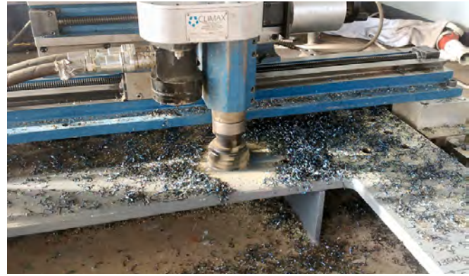
Onsite milling of a support base to a known Datum
