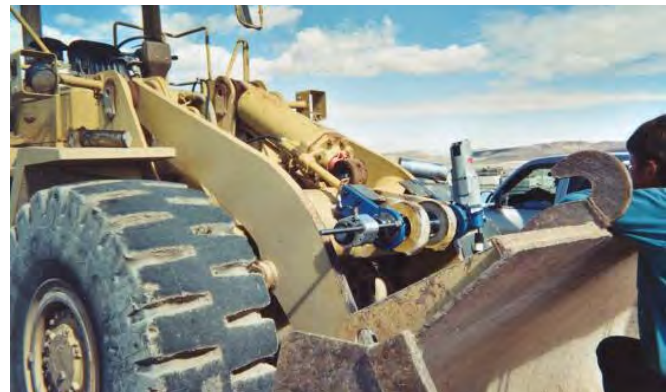
Line Boring of a Digger Bucket Pivot Point
