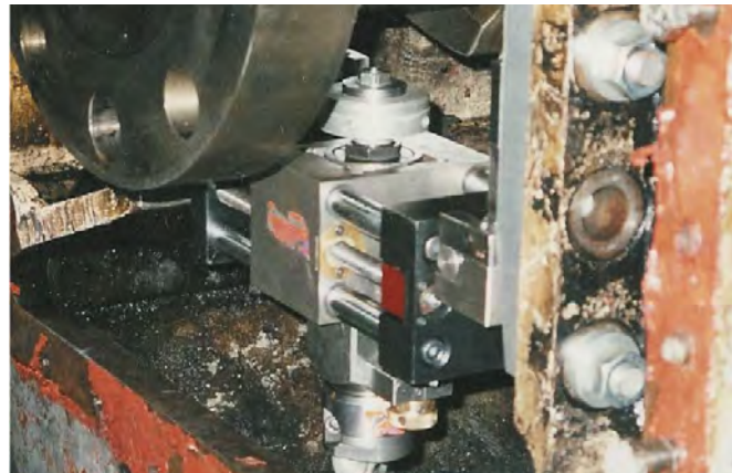
Mounting the "Millgrind" Equipment on a 400mm Ø Main Journal
