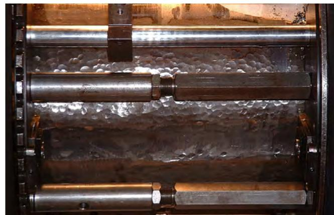
Crankshaft Straightening (Peening)
