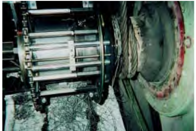
The same 300mm \varnothing Fanshaft Journal During Machining
