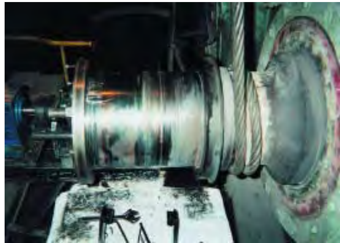
A Badly Worn 300mm \varnothing Fanshaft Journal Prior to Any Machining Work
