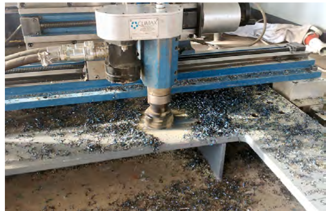
On Site Milling of a Weapon Support Base
