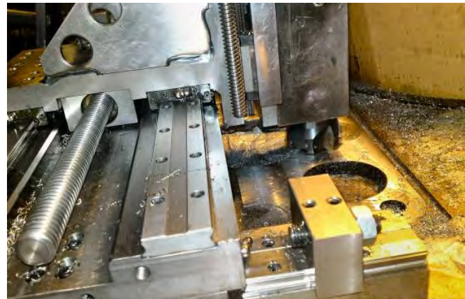
On Site Milling of a Diesel Engine Entablature Base
