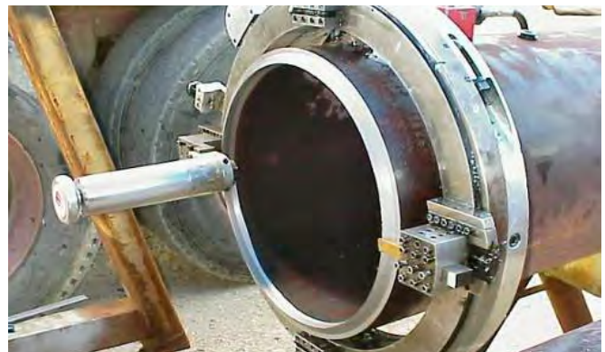
Pipe bores and outside diameters machined to suit matching pipe work
