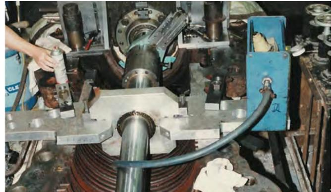
Setting Up the Boring bar to machine Turbine Axial and Radial Seals
