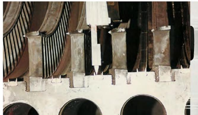
Machining to give Correct clearances on the Seal strips
