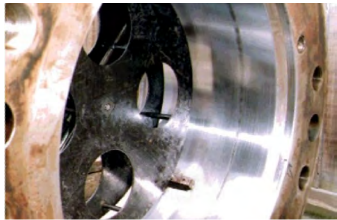
Internal Honing of a 900mm Ø Tailshaft Bearing Internal
