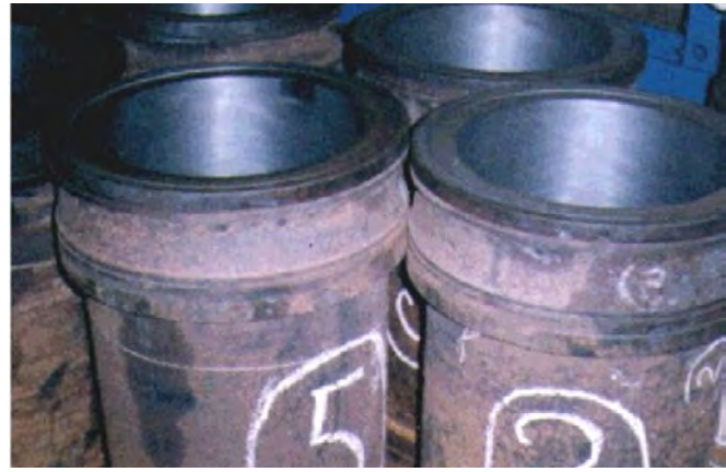
Internally Honed 400mm Ø Cylinder Liners
