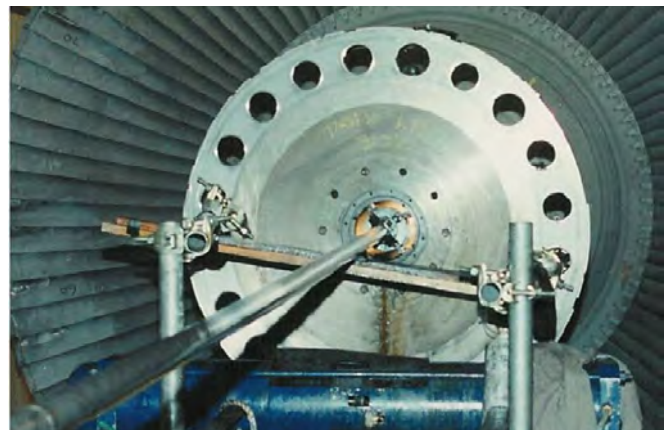
Internal Honing of a 110 mm Ø 4 Metre long Turbine Rotor Bore
