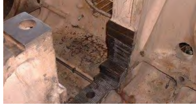
Main Bearing Pocket Section Removed
