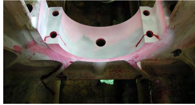
Damaged Main Bearing Cap Stud Hole
