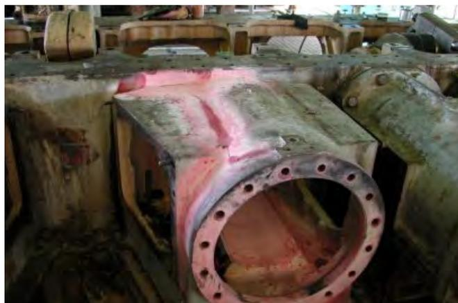
Removing & Inserting a Complete Top Section due to cracks
