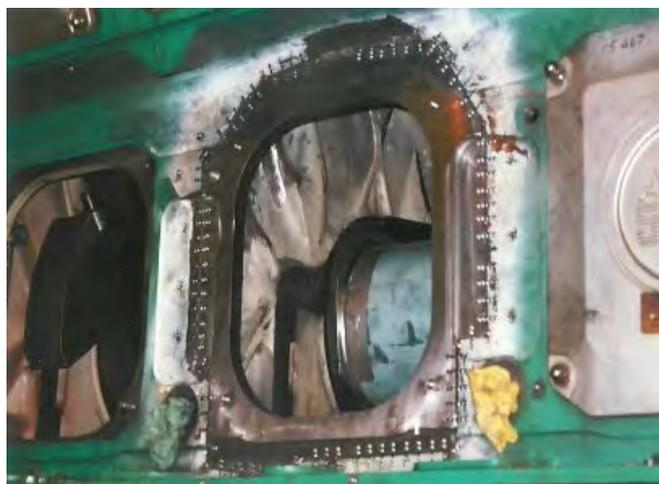
Removing a Damaged Diesel Engine Door And Metal Stitching In A New Insert
