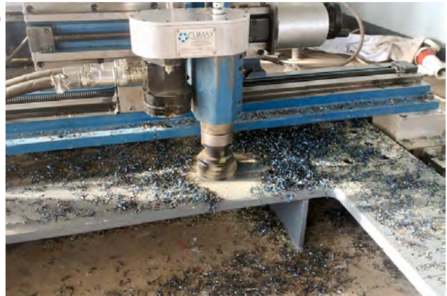
On Site Milling Of A Weapon Support Base
