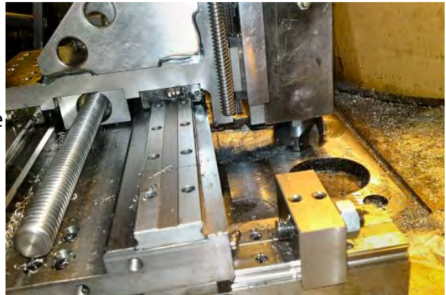
On Site Milling Of A Diesel Engine Entablature Base
