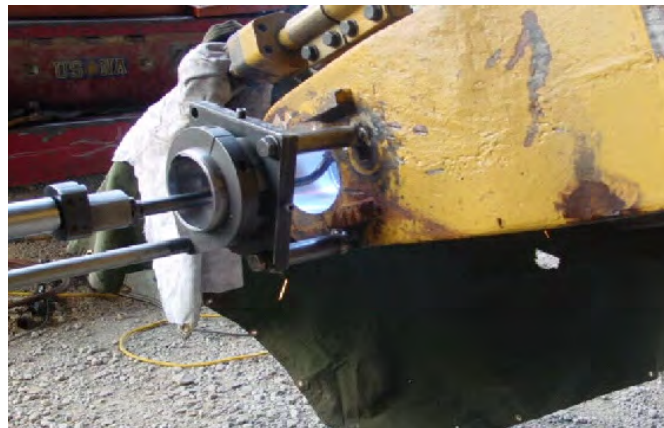
Orbital Welding Of A 100mm Ø Bore On a Digger Bucket
