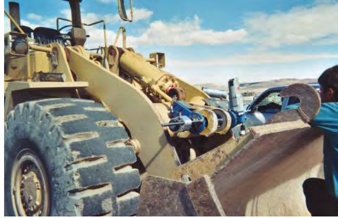
Line Boring A Set Of Digger Bucket Pivot Bearings Approx 60mm Ø
