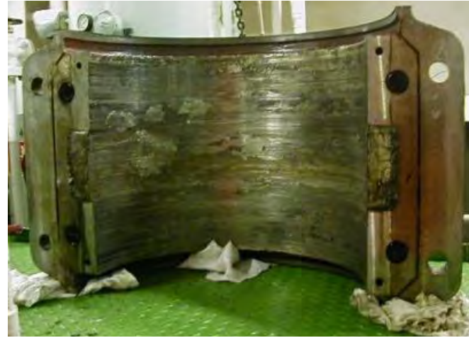
Damaged White Metal Bearing
