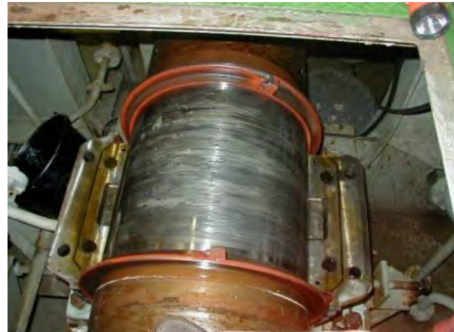
Damaged 505mm Ø Tailshaft Journal
