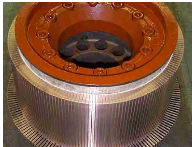
An Example of a Machined Commutator
