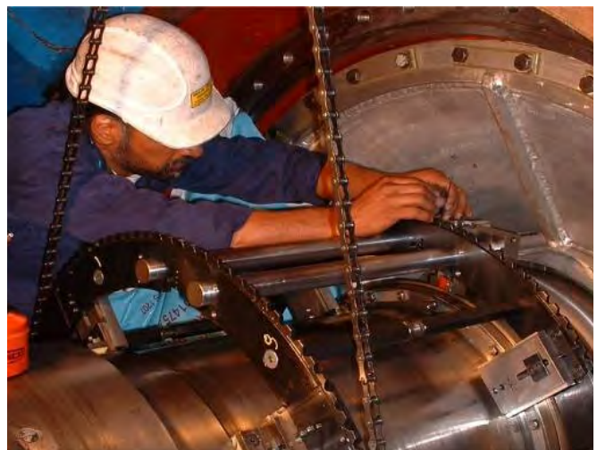
Machining and Polishing of a 610 mm Ø Hydrogen Seal Face
